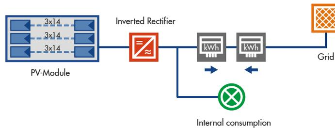
The generator of a photovoltaic-system consists out of a corresponding amount of photovoltaic modules according to the demand to be produced which are producing the necessary energy for feeding the local electric supply networks as well as providing the internal consumption. This energy generated by solar radiation is now converted into a compatible voltage waveform for the grid.
